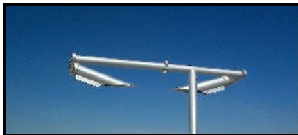
Figure 5.- Frontal dispersion measurer.
