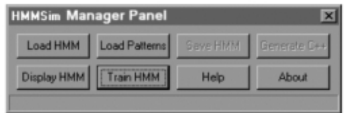
Fig. 1. Manager panel showing the functionality of HMMSim (loading a HMM, opening a training window, loading training patterns, displaying a HMM, saving a HMM, generating C++ code for a trained HMM and receiving help about the tool).
